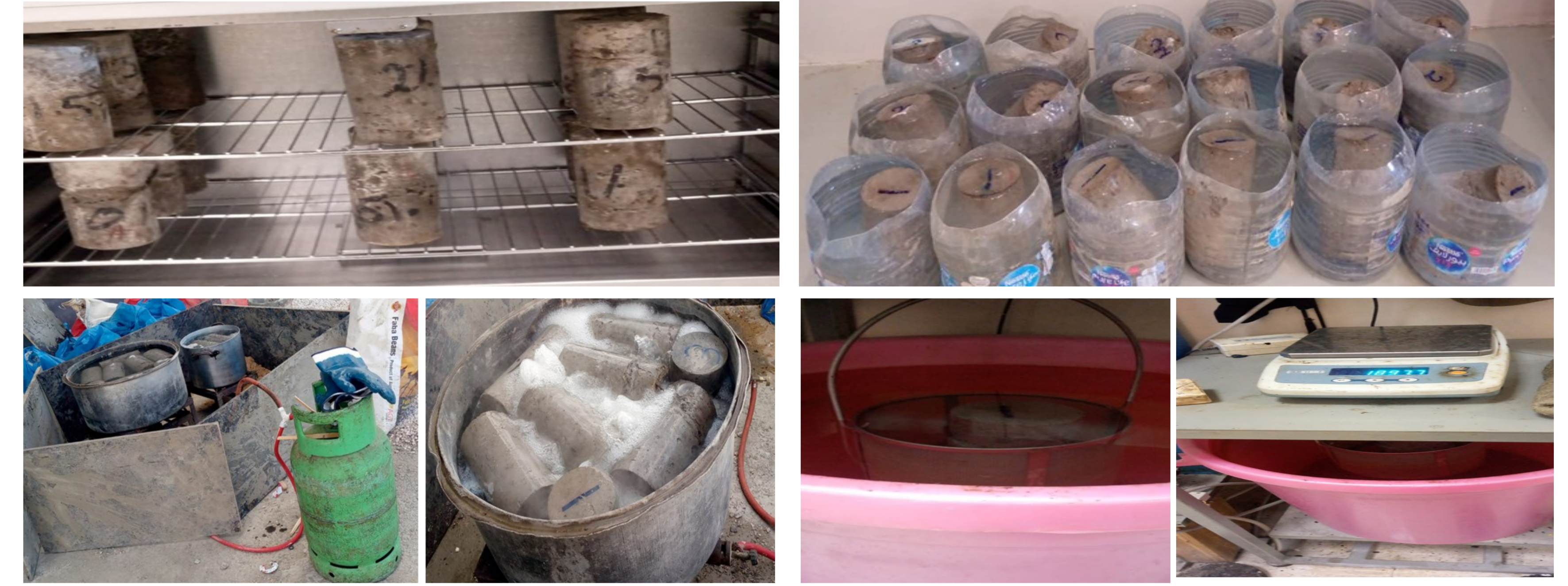
Fig5. Density, Absorption% and void % process.
