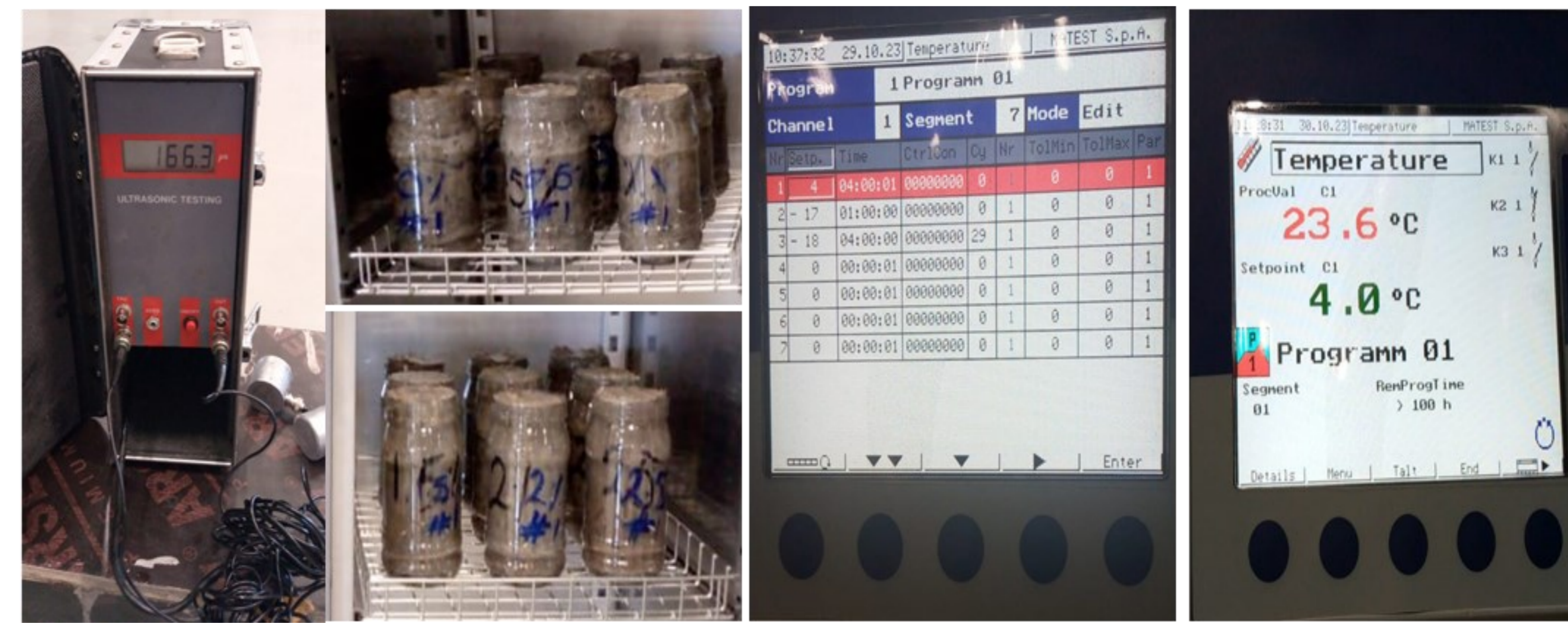
Fig5. Main phases at resistance of concrete to rapid freezing and thawing process.
