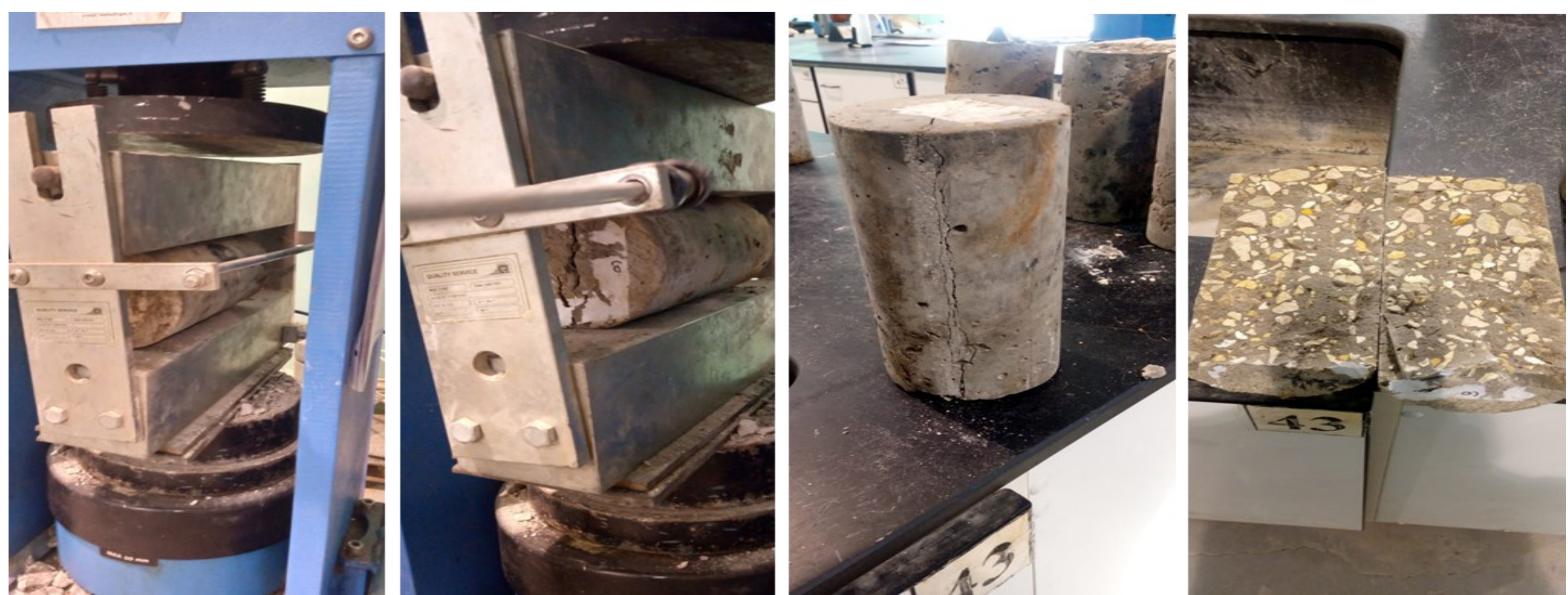
Fig7. Splitting tensile test process
